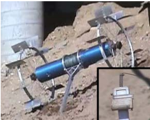
Fig. 4. Axel taking a sample by pointing the caster arm into the ground and turning in place. Sand enters through the openings on the ends of the removable sampling tubes (inset).
