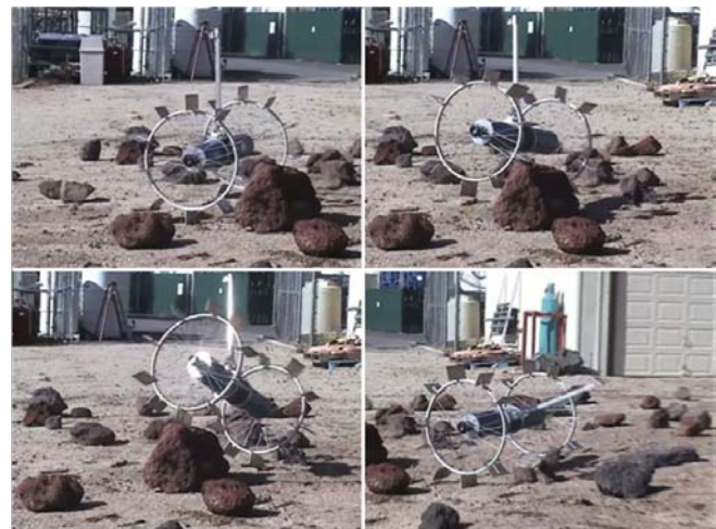
Figure 14 – From top-left to bottom right: Axel uses its large radius paddle wheels to traverse over a rock more than half of its wheel diameter in the JPL Mars Yard.
