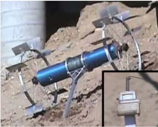
Figure 4 – Axel taking a sample by pointing the caster arm into the ground and turning in place. Sand enters through the openings in the ends of the removable sampling tubes (inset).
