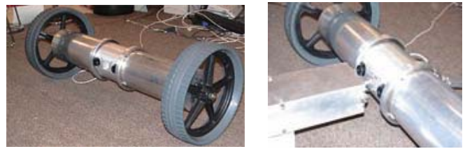
Figure 12—Original Axel (left), Axel docking to a payload module (right)
