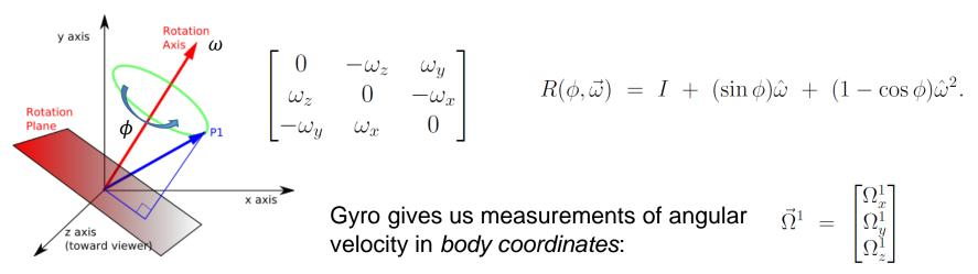
$$R_{WB}(t_{k+1}) = R_{WB}(t_k)e^{\Delta\phi(t_{k+1})\hat{\omega}(t_{k+1})}$$
