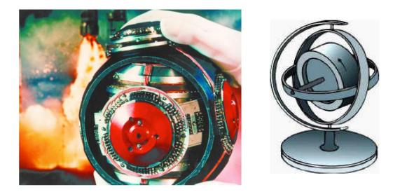
**Mechanical Gyro:** A spinning wheel will resist any change to its angular momentum vector. Maintains constant orientation if in a frictionless gimbal
