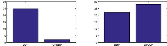
Fig. 4: Comparison of DDP and GPDDP for the six-link arm task. Left figure: time consumed at each iteration for linearization (sec). Right: number of iterations to obtain the optimized trajectory.
