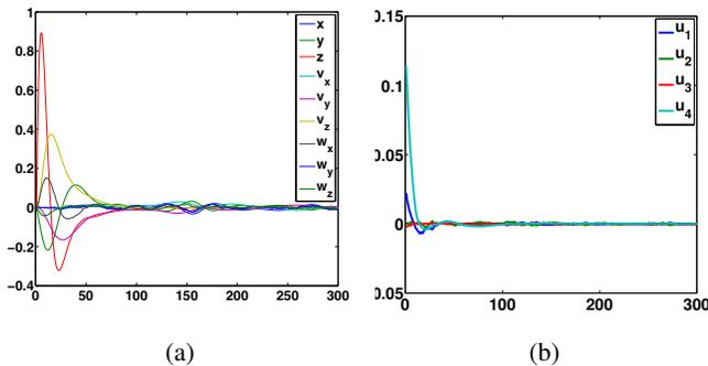
Fig. 5: Simulation results for the helicopter hovering task. In all plots, the X-axis is the time steps. (a) optimized state trajectories. (b) optimal controls.
