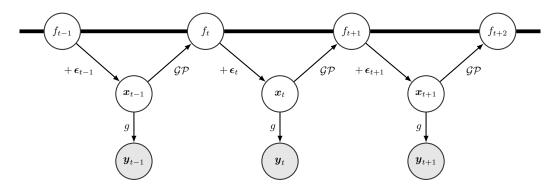
Figure 4.15: Graphical model of a Gaussian Process state space model. The random variables f represent the GP function values, which are fully connected to each other, as represented by the thick line. The transition of  $\mathbf{x}_{t-1}$  to  $\mathbf{x}_t$  is modelled by the GP followed by the addition of process noise  $\epsilon_t$
