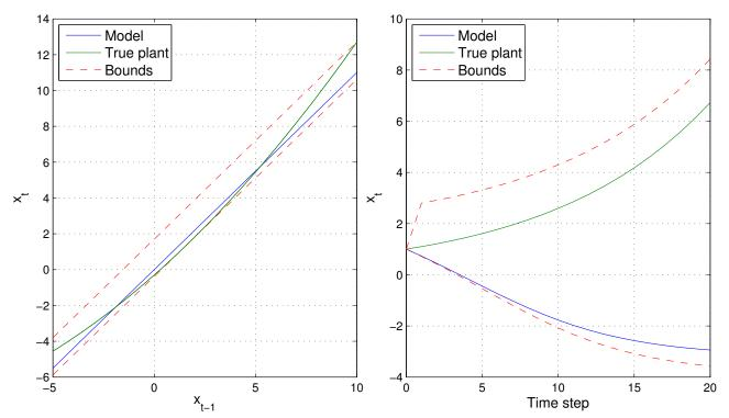
Figure 4.1: Illustration of the effect of model errors on trajectory prediction. The left plot shows the true nonlinear transition function in green and the linear model of the plant in blue. Whilst these look visually similar they lead to very different trajectories as shown in the right hand plot. In order to capture the true trajectory in a predicted set by considering perturbations to the linear model's offset parameter we would need to use all models within the red dashed lines.
