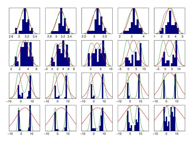
Figure 4.10: Distributions over the pendulum angle as it falls from upright over 20 time steps. The first plot in the top left corner shows the initial distribution over start positions. The histogram shows the true distribution from thirty repeats, the red Gaussians show the predicted distributions using Gaussian moment-matching at each time step, the green lines show a kernel-smoothed density estimate from the particle simulation method.
