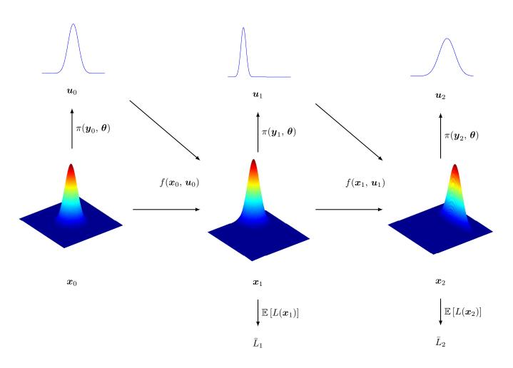
Figure 4.3: An illustration of the plant simulation step under a control policy  $\pi$ , for a 2D system with 1 control variable and 2 time steps.
