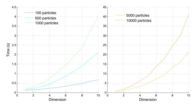
Figure 3.30: Wall clock times for the Particle Filter algorithm to compute the marginal likelihood estimate and its gradient using varying numbers of particles on systems with dimension ranging from 1 to 10. The data set consisted of a single observed trajectory of length 20 time steps.
