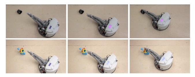
Figure 4.7: A series of photos demonstrating the optimised policy in action on the mobile robotic arm from Bischoff et al. (2014). The robot approaches the item, extends the arm and manipulates the claw so as to successfully pick up the object.
