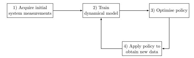
Figure 4.2: Diagram of the high level steps of the control learning framework. Once we have some initial data we can train a dynamical model and optimise the control policy. From this point we can collect more data and then iterate the procedure to improve the dynamical model and control policy.
