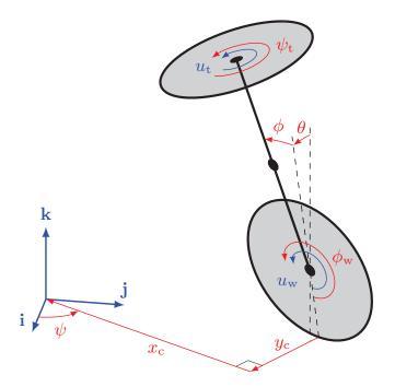
Figure 1.10: Idealised diagram of the unicycle. The state is described by the pitch  $\phi$ , roll  $\theta$ , and yaw  $\psi$  angles, the angles of the wheel  $\phi_w$  and flywheel  $\psi_t$ , and their corresponding time derivatives. In addition there are two position variables, which map the position of the origin w.r.t. the unicycle (self-centred coordinates)  $x_c$  and  $y_c$ . Figure reproduced from Hall (2013).
