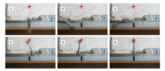
Figure 4.4: A series of stills from a video of a control policy successfully swinging up the pendulum.
