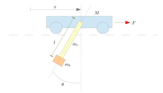
Figure 1.9: The cart and pendulum system. A cart of mass M is free to move in one dimension under the action of a force F. Attached to the centre of the cart is a pendulum, consisting of a rod of mass  $m_r$  and length l, and a bob of mass  $m_b$ . The pendulum is unactuated and free to rotate about its attachment. The distance of the cart from the origin in denoted by x and the angle of the pendulum by  $\theta$ .
