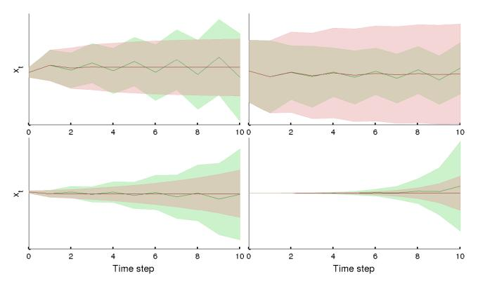
Figure 4.14: Comparison between simulations of a 1D uncertain linear system with (green) and without (red) the covariance between the state and the model parameters. The four plots show simulations using four different randomly generated 1D systems over a horizon of 10 steps. The solid line shows the mean of the state distribution and the shaded region  $\pm 2$  standard deviations.
