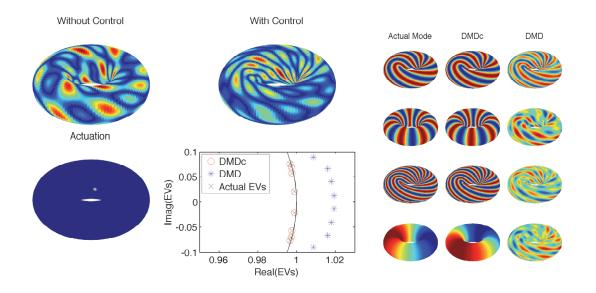
**Figure 3.** The top left panel illustrates one realization of Example 3 without actuation over time. The right panel illustrates the same dynamical system but with actuation. The bottom left panel illustrates the actuation applied in the spatial domain. The bottom middle panel shows a comparison between the actual eigenvalues and the eigenvalues found from DMD and DMDc. On the right the first four dynamic modes of DMD and DMDc are compared to the actual underlying spatial modes.
