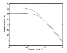
**Figure 2.** The singular values of the frequency response for a large-scale stable linear system. The blue line is from the model from DMDc, and the red is from the real model. Note that an equivalent frequency response cannot be constructed from DMD alone since it does not consider input-output systems.
