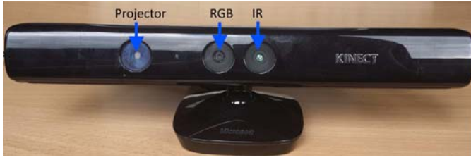
Fig. 2. Sensor placement within a Kinect SL camera. The baseline is of approximately 7.5 cm.
