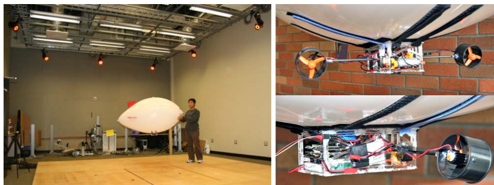
Fig. 2 The left image shows the blimp used in our test environment equipped with a motion capture system. It has a customized gondola ( right images ) that includes an XScale based computer with sensors, two ducted fans that can be rotated by 360 degrees, and a webcam
