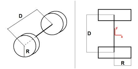
The left view is an isometric view and the right view is an overhead view of the same robot. The origin of the robot is indicated by the crosshair (midway between the two wheels, and slightly above the ground).
