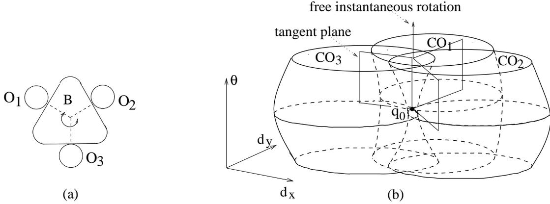
Figure 6.2: (a) A 3-finger equilibrium grasp of a triangular object. (b) The finger c-obstacles completely surround the object's configuration point  $q_0$ .
