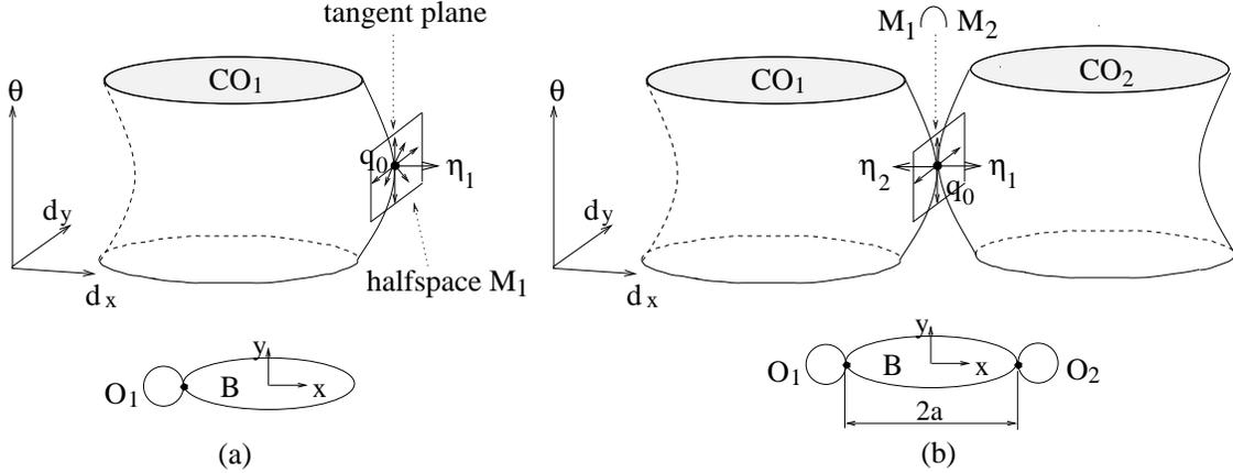
Figure 6.1: (a) The halfspace  $M_1$  approximating the exterior of  $\mathcal{CO}_1$  at  $q_0$ . (b) The 1<sup>st</sup>-order approximation to the free motions,  $M_1 \cap M_2$ , at a two-finger equilibrium grasp.
