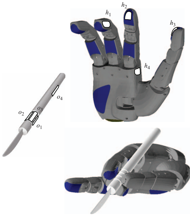
Fig. 1. A typical grasp configuration for a scalpel can be specified by requiring the contact of regions h_1, \dots, h_4 of the hand, with regions o_1, \dots, o_4 on the object (top). The configuration problem is to determine how should the hand be configured relative to the object, in order to bring the hand regions into contact with their corresponding object regions (bottom).
