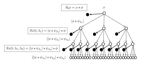
Fig. 4. A scattering transform iterates on wavelet modulus operators  $|W_m|$  to compute cascades of m wavelet convolutions and moduli stored in  $U_m x$ , and to output averaged scattering coefficients  $S_m x$ .
