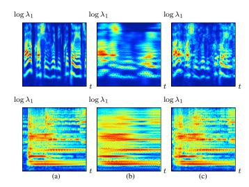
Fig. 5. (a): Scalogram  $\log |x\star\psi_{\lambda_1}(t)|$  for recordings of speech (top) and a cello (bottom). (b,c): Scalograms  $\log |\widetilde{x}\star\psi_{\lambda_1}(t)|$  of reconstructions  $\widetilde{x}$  from first-order scattering coefficients (l=1) in (b), and from first- and second-order coefficients (l=2) in (c). Scattering coefficients were computed with  $T=190~\mathrm{ms}$  for the speech signal and  $T=370~\mathrm{ms}$  for the cello signal.
