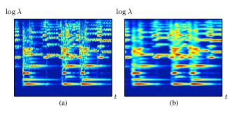
Fig. 2. (a): Scalogram  $\log |x\star\psi_\lambda(t)|^2$  for a musical signal, as a function of t and  $\lambda$ . (b): Averaged scalogram  $\log |x\star\psi_\lambda|^2\star\phi^2(t)$  with a lowpass filter  $\phi$  of duration T=190 ms.
