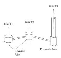
Figure 1: Cylindrical Manipulator
