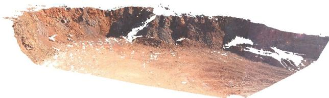
Fig. 3. Laser Scanner data set taken at Mt. Tom Price mine in Western Australia using a RIEGL LMSZ420. The data set consists of over 1.85 million data points. The data set spanned about 135 x 72 sqm.
