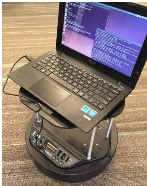
Figure 1: TurtleBot 2 based on the Kobuki platform
