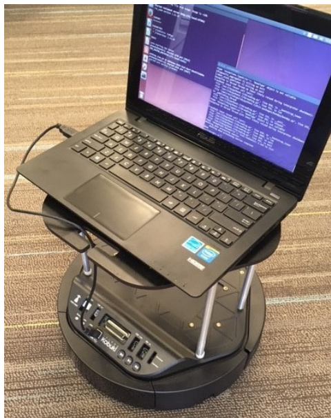
Figure 1: TurtleBot 2 based on the Kobuki platform
