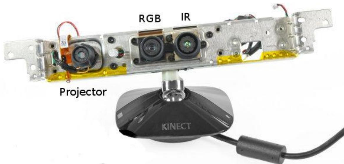
Figure 2: The Microsoft Kinect with the cover taken off. Source: [http://www.ros.org/wiki/kinect\\_calibration/technical](http://www.ros.org/wiki/kinect_calibration/technical)
