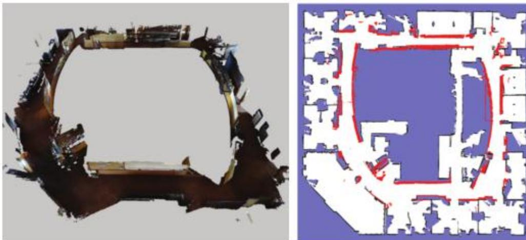
Figure 6: A map created with Henry et al.'s RGB-D Mapping framework (left), and the corresponding ground truth (right) (Henry et al. 2012).
