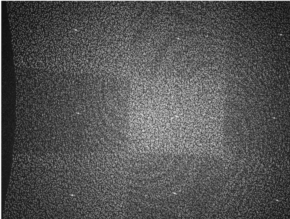
Figure 1: MS Kinect infrared pattern. Source: [http://www.ros.org/wiki/kinect\\_calibration/technical](http://www.ros.org/wiki/kinect_calibration/technical).
