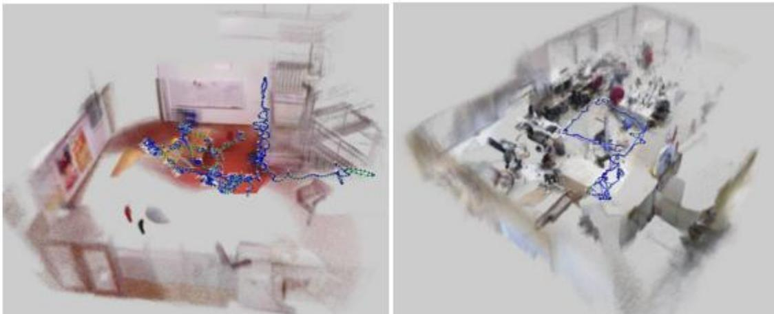
Figure 10: Point cloud maps created by the algorithm, with the trajectories of the MAV shown (Huang et al. 2011).
