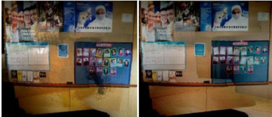
**Figure 7: comparison of data in a point cloud representation (left, 56.6 million points) and the surfel representation used by the RGB-D Mapping framework (right, 2.2 million surfels) (Henry et al. 2010).**
