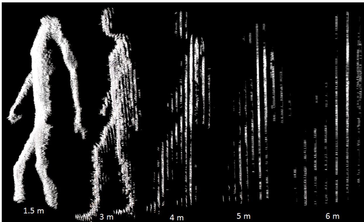
Figure 5: Depth data of a mannequin captured from the front and shown from the side. From left to right, the mannequin is shown as captured at 1.5 m, 3 m, 4 m, 5 m, and 6 m.
