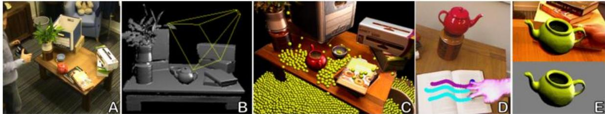
Figure 14: KinectFusion. A) user holding a Kinect. B) reconstructed 3D model with camera pose. C) texture-mapped model with simulated particles. D) touch interaction example. E) object segmentation (Izadi et al. 2011).
