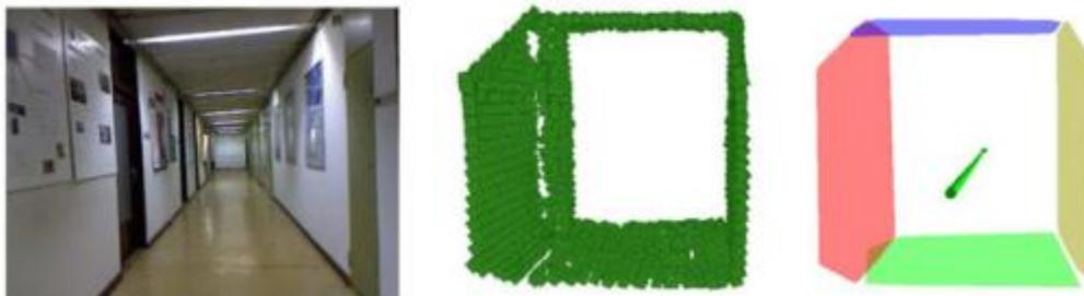
Figure 11: Plane estimations from Lange et al.’s MAV (Lange et al. 2012).
