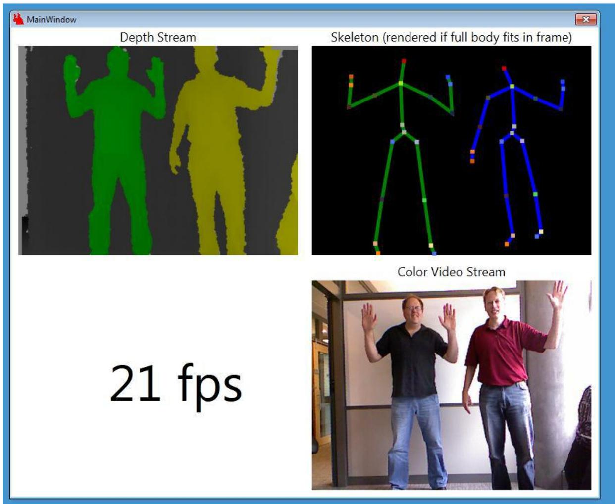
Figure 16: A screenshot of the SkeletalViewer application included in the Microsoft Kinect SDK (source: SkeletalViewer Walkthrough, Microsoft Kinect SDK).
