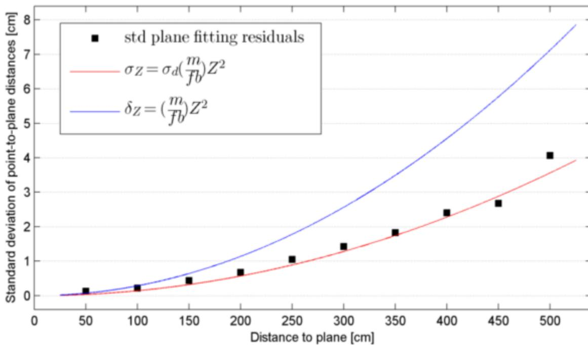
Figure 4: Microsoft Kinect depth resolution vs. depth (Khoshelham & Elberink 2012). Theoretical random error is shown in red (bottom curve), while the theoretical resolution is shown in blue (top curve).
