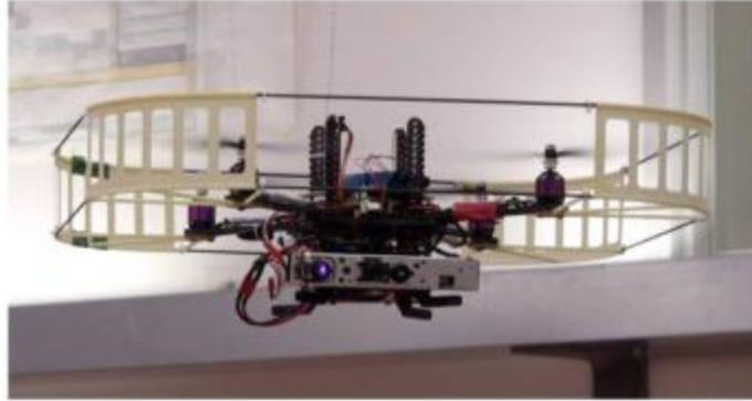
Figure 9: Autonomous micro air vehicle (MAV) used with an RGB-D sensor mounted at the front (Huang et al. 2011).
