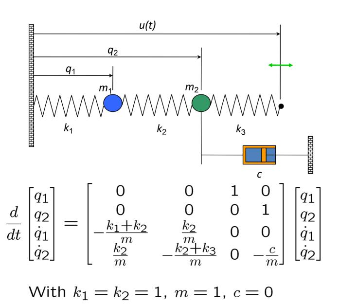
$v_{1,2} = \begin{vmatrix} 1\\ \pm 1i\\ \pm 1i \end{vmatrix} \qquad v_{3,4} = \begin{vmatrix} -1\\ \pm \sqrt{2}i\\ \pm \sqrt{2}i \end{vmatrix}$
