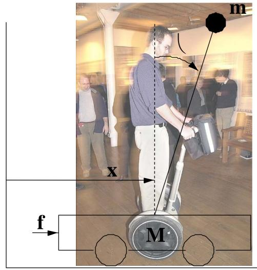
$(M+m)\ddot{x} + ml\cos\theta\ddot{\theta} = -b\dot{x} + ml\sin\theta\dot{\theta}^2 + f$  $(J+ml^2)\ddot{\theta} + ml\cos\theta\ddot{x} = -mgl\sin\theta$
