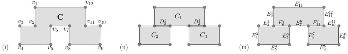
Fig. 2. (i) an example of a two dimensional configuration space  $\mathbf{C}$  (shown as a shaded region) where  $\mathbf{v}_1, \mathbf{v}_2, \dots, \mathbf{v}_{12}$  are its 0-faces. (ii) and (iii) the structure induced from  $\mathbf{C} = C_1 \cup C_2 \cup C_3$ . In this situation, observe that  $D_2^1$  and  $D_3^1$  are exactly  $E_6^2$  and  $E_{11}^7$ , respectively.
