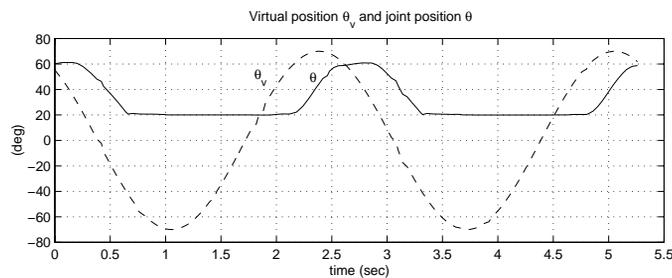
Fig. 8. Desired and real position of the finger.
