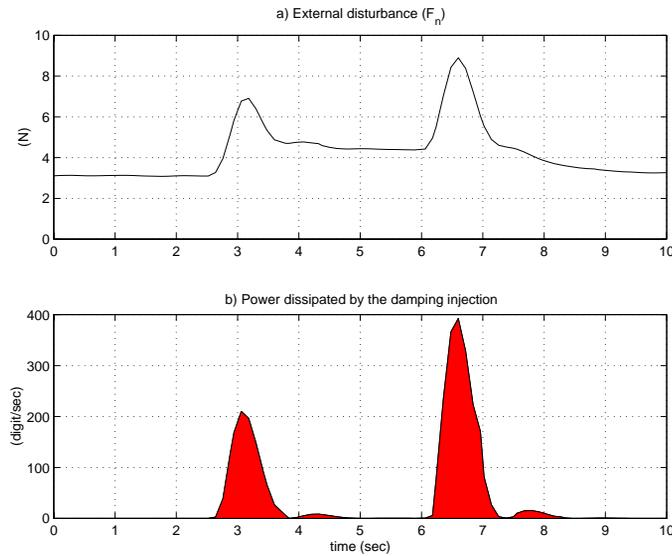
Fig. 12. External disturbance applied during the grasp (a) and relative dissipated energy for achieving stability (b).
