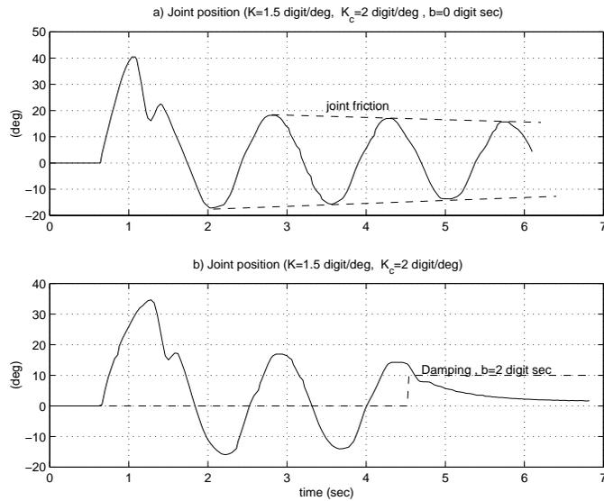
Fig. 7. Stability of the control loop without (a) and with (b) damping.
