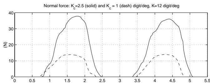
Fig. 9. Forces applied to the obstacle with two different values of  $k_c$ .
