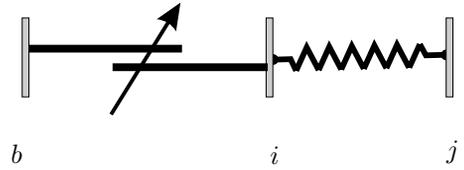
Fig. 3. Schematic drawing of a power consistent variable spring.
