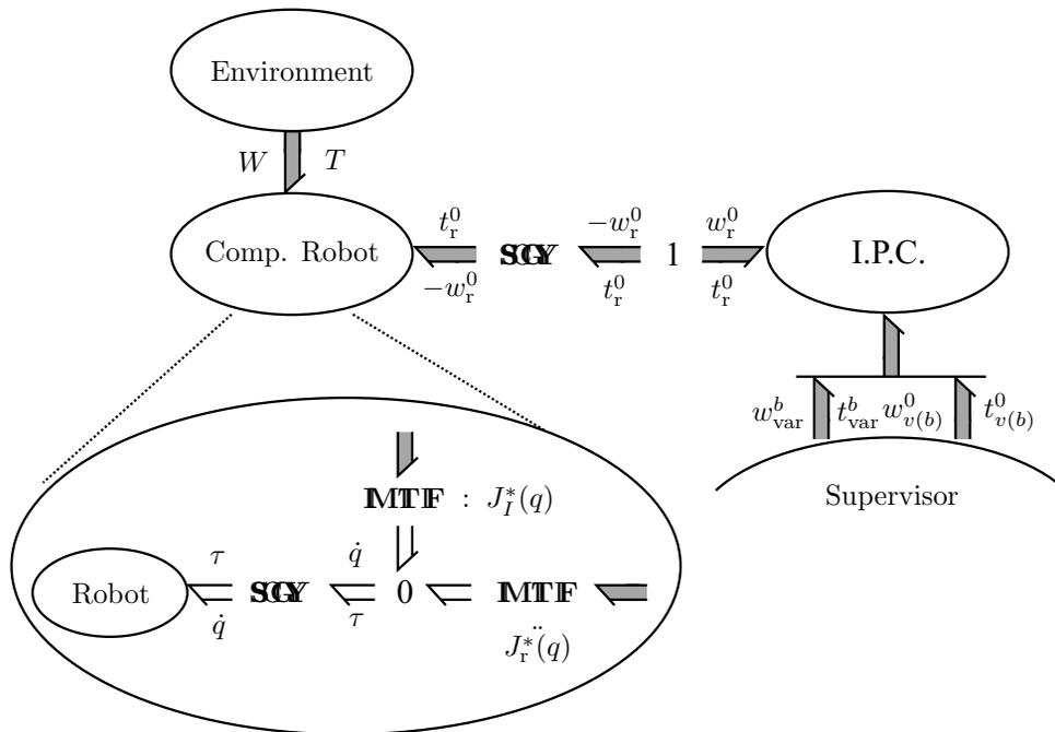
Fig. 4. The interconnection between the robot and the intrinsically passive controller.
