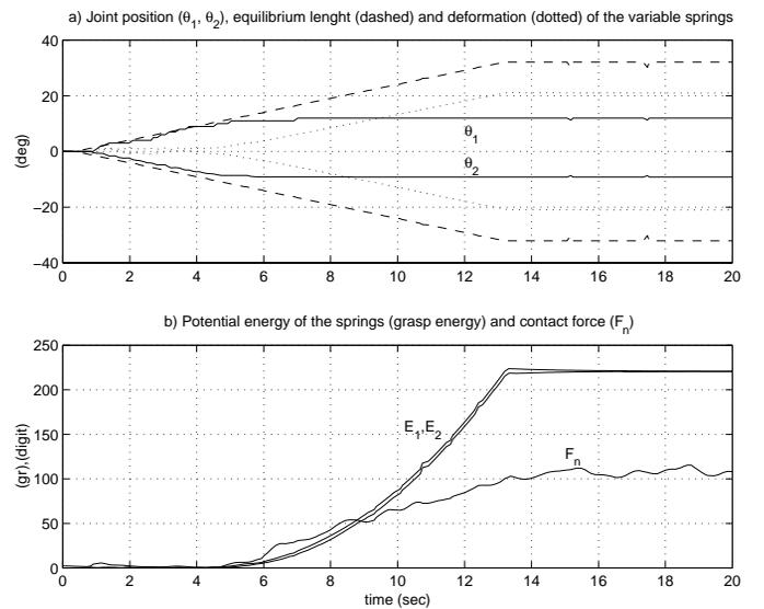
Fig. 10. Result of a grasp task: (a) Joint positions, springs' equilibrium length and deformations; (b) potential energies and contact force.
