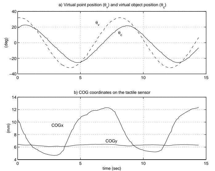
Fig. 11. Desired (dashed) and computed (solid) position of the virtual object (a); Contact point (COG: center of gravity) position on the tactile sensor (b).
