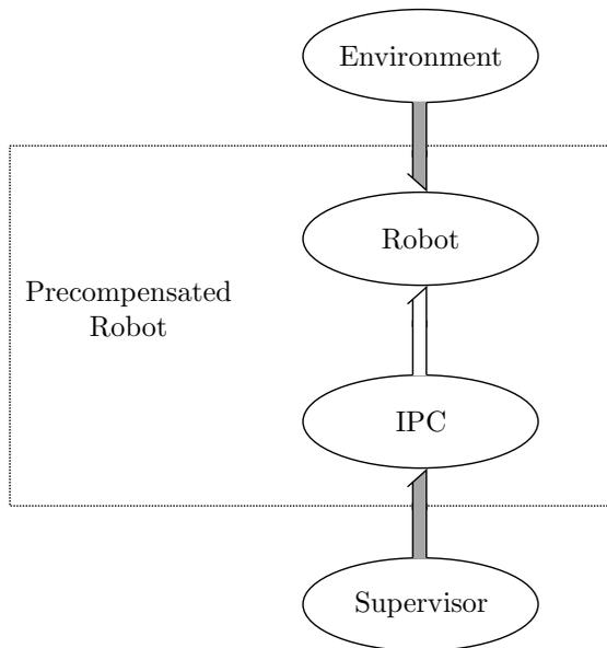
Fig. 1. The general form of an intrinsically passive control scheme.
